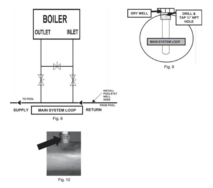
Note: The drawings and instructions above show only one of several acceptable ways of installing the dry well into main system loop. The use of saddle clamps and "Weld O Lets" (shown in Fig. 10) are acceptable. Follow clamp manufacturer's instructions.
